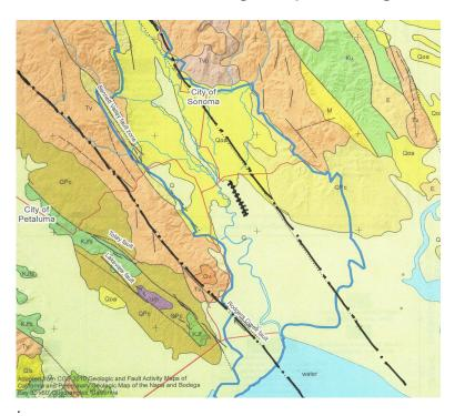
The USGS geologic map above shows the tanker yard (hatched line) as it iocated between the Eastside Fault to the east and the Rodgers Creek Fault to the west (chain-link lines).
